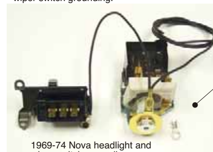
1968 Nova headlight and wiper switch grounding.
