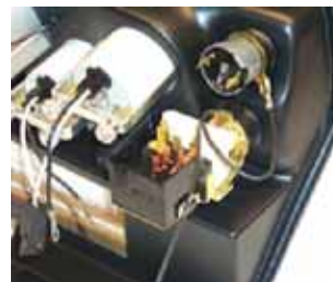
1968 Nova headlight and wiper switch grounding.
